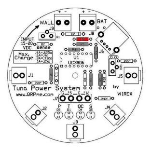
A 150K blue bodied 1% resistor (Brown-Green-Black-Orange-Brown) is installed at location R4.
