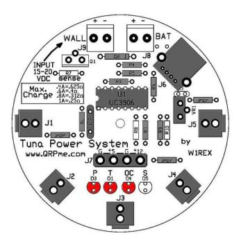
The 3 LEDs are installed at locations D1, D3 and D4. D1 = Red, D3 = Green & D4 = Orange. The short LED lead is inserted into the hole marked by the flat section on the silk screen.
