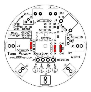
Start with three 1K resistors (Brown-Black-Red) resistors at positions R1, R2 and R9.
