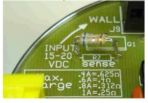
you have different size batteries you will be charging, configure the sense resistor for the smallest battery size. Better to take a little longer to charge the bigger
