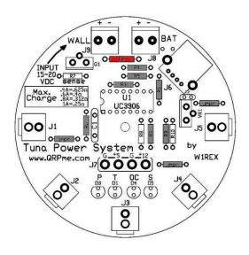
Install a 1N4004 diode at location D1. Be sure to orient the striped end of the diode with the hole as indicated by the silk screen.
