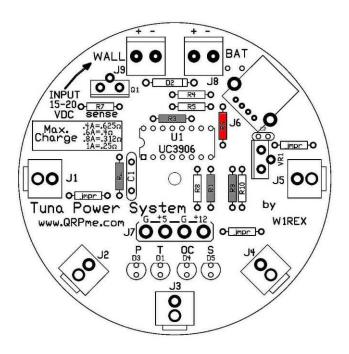
Now install a 33K 1% resistor (Orange-Orange-Black-Red-Brown) blue bodied resistor at position R6.
