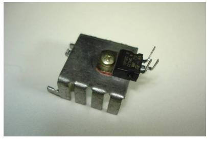
Mount the heat sink to Q1 (marked TIP32C) and bend the leads like the
