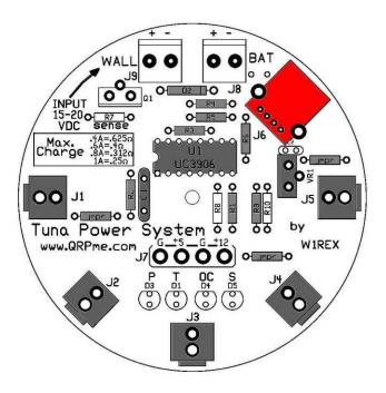
The USB connector is installed at location J6. Have the end of the connector nearest the edge of the board slightly raised in the air before soldering.
