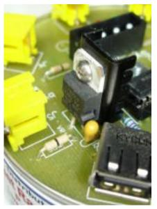
The 5 yellow RCA connectors are now installed at positions J1 through J5.
