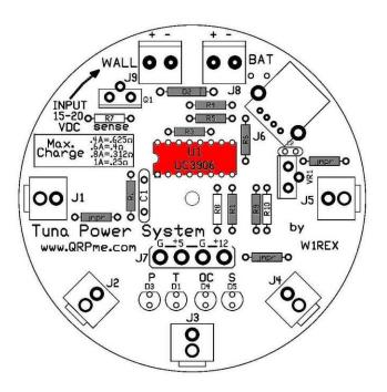
Now you can install the 16 pin socket for U1. Orient the indented end of the socket to align with the indentation indicated by the silk screen.
