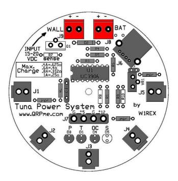
Install the 2 screw terminal connectors at locations J8 & J9 with the wire entry locations oriented towards the outside of the board.
