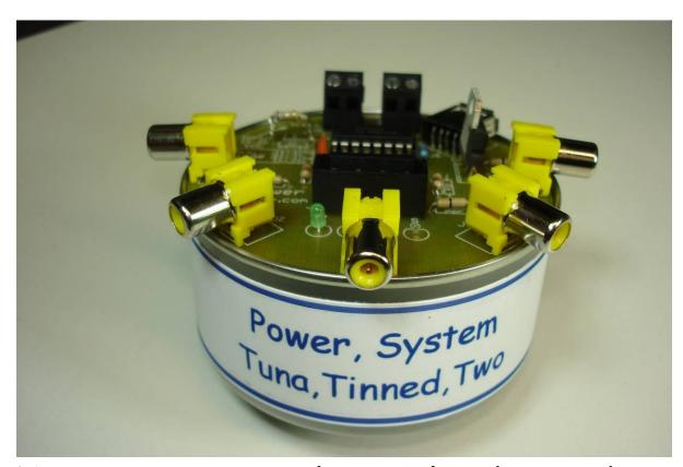
Now you can mount the completed printed circuit board to the can using the supplied nut and bolt. The bolt is inserted through the hole in the bottom of the can and then the board. The nut is installed on the top. Do not over tighten.
