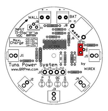
A 5 volt regulator (marked L7805) with small heat sink is installed at location VR1.
