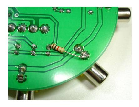
R10, a 1K ohm (Brown-Black-Red) resistor is relocated to the bottom of the board. Solder it to the top pad of LED D2 to the outside
